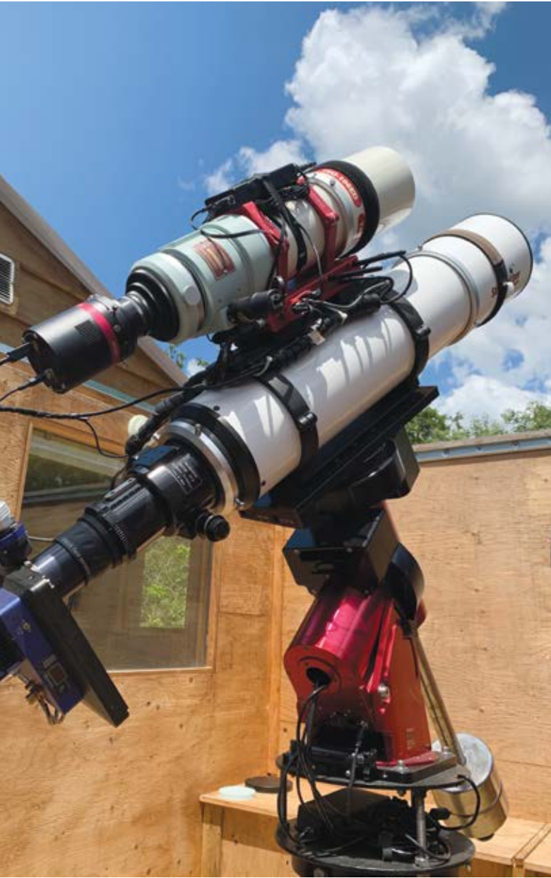
▲ TWO “EYES” ON THE SKY Canadian astrophotographer Ron Brecher gets nearly twice as much exposure time with every target by piggybacking a Takahashi FSQ-106ED astrograph atop a Sky-Watcher Esprit 150 triplet apochromatic refractor. The larger scope images with a monochrome QHY16200A CCD camera, while the smaller FSQ records the same field with a QHY367C Pro color CMOS camera.
