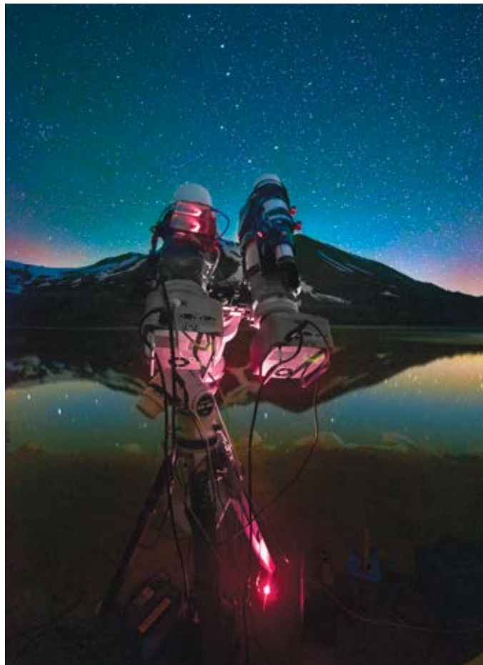
▲ TANDEM MOUNTING Another mounting option is to install both telescopes on a tandem platform. As seen here, imager Rogelio Bernal Andreo uses a pair of Takahashi FSQ-106 astrographs with two SBIG STL-11000M CCD cameras. Typically, he uses one scope to record color-filtered images while the other collects filtered luminance.
